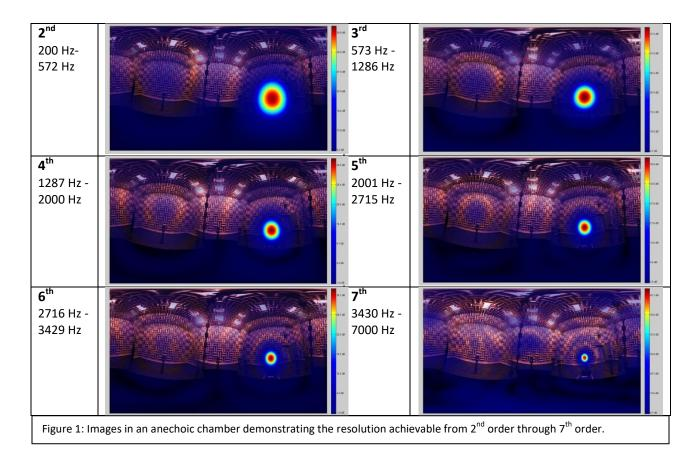
The following chart contains the angular beam width for each order and the corresponding physical widths for the following distances 1, 2, 5, 10, and 20. You can use any units you want here.
