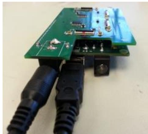
Once the chains have all been connected to the hub board and the software has been successfully installed you can connect the USB cable and power cable to the hub board. You should receive a message that it is installing drivers for the xem3010 FPGA unit. Once this has completed you should be able to capture data from the array using the command line interface described below.
