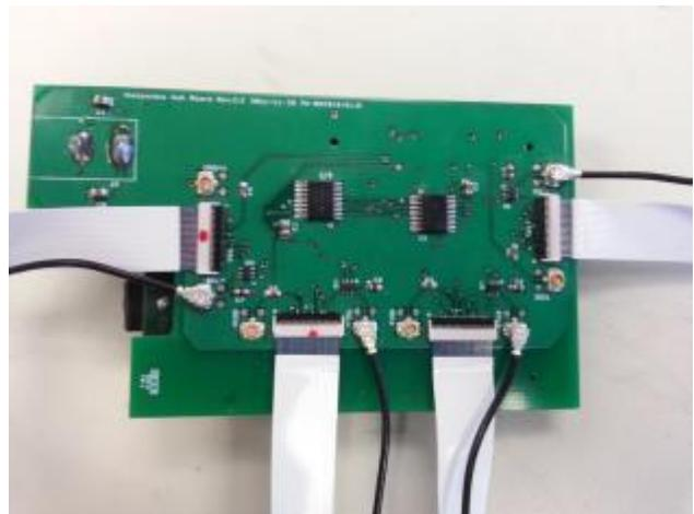
Connecting microphone to microphone, cables will link “J2-TOSTR” to “J1-TOHUB” connectors. Ensure that “J2-TOSTR” connects down the chain away from hub. First Microphone closest to hub will have “J1-
